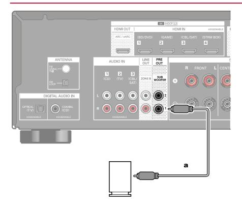
Connect a powered subwoofer with this unit using a subwoofer cable.
