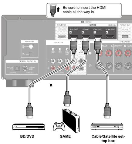
This is a connection example of an AV component equipped with an HDMI jack. When connecting with an AV component that conforms to the CEC (Consumer Electronics Control) standard, you can use the HDMI CEC function(\*) that enables linking with input selectors, etc. and the HDMI Standby Through function that can transmit video and audio signals of the AV component to the TV even if this unit is in standby mode.
