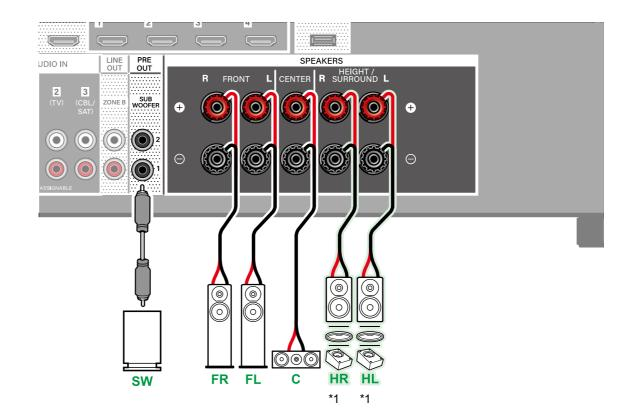
\*1 Connect the Height Speakers you have actually installed (HL/HR: Height Speakers, Top Speakers, Dolby Enabled Speakers).
