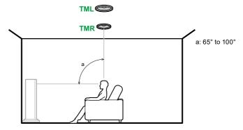
**TML**, **TMR** Fit top middle speakers on the ceiling directly above the listening position.
