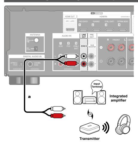
By connecting an Integrated Amplifier to the ZONE B LINE OUT terminal, you can play the same source in the other place (ZONE B) as in the main room. Also, when you connect a transmitter for wireless headphones or wireless speakers, you can play audio through these devices.
