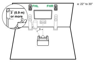
**FHL**, **FHR** Place the front high speakers directly above the front speakers, angled to face the listening position.
