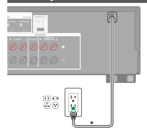
Connect the power cord after all the connections are completed.
