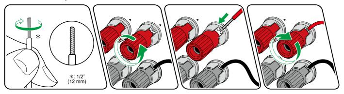
Make correct connection between the unit's jacks and speaker's jacks (+ side to + side, and - side to - side) for each channel. If the connection is wrong, a bass sound will not be reproduced properly due to reverse phase. Twist the wires exposed from the tip of the speaker cable so that the wires do not stick out of the speaker terminal when connecting. If the exposed wires touch the rear panel, or the + side and - side wires touch each other, a malfunction may occur.
