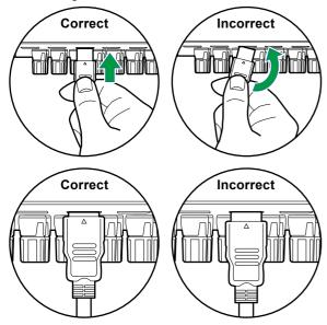
Hold the terminal housing on the HDMI cable when unplugging. Pulling on the cable may lead to damaged cabling.
