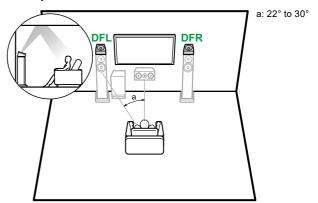
**DFL**, **DFR** The Dolby enabled speakers (front) are installed on top of the front speakers.
