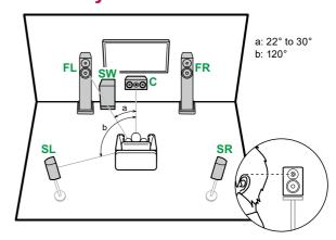
FL, FR Place the Left and Right Front Speakers to match ear height.C The center speaker should be set up facing the listening position at
